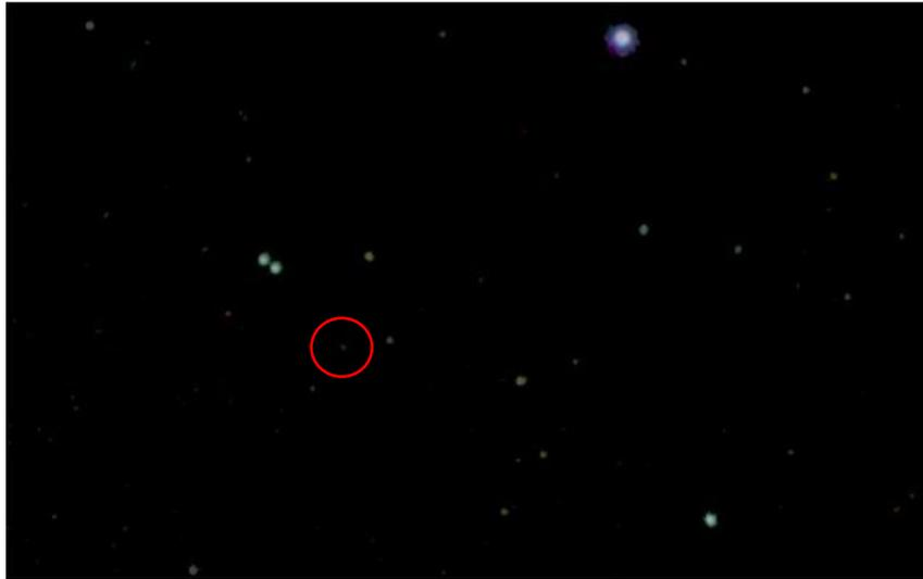
Result of image processing from Ximea camera during ground test. Red circle shows the weakest star with magnitude 9.15, recovered by post-processing from time series of noised images.
