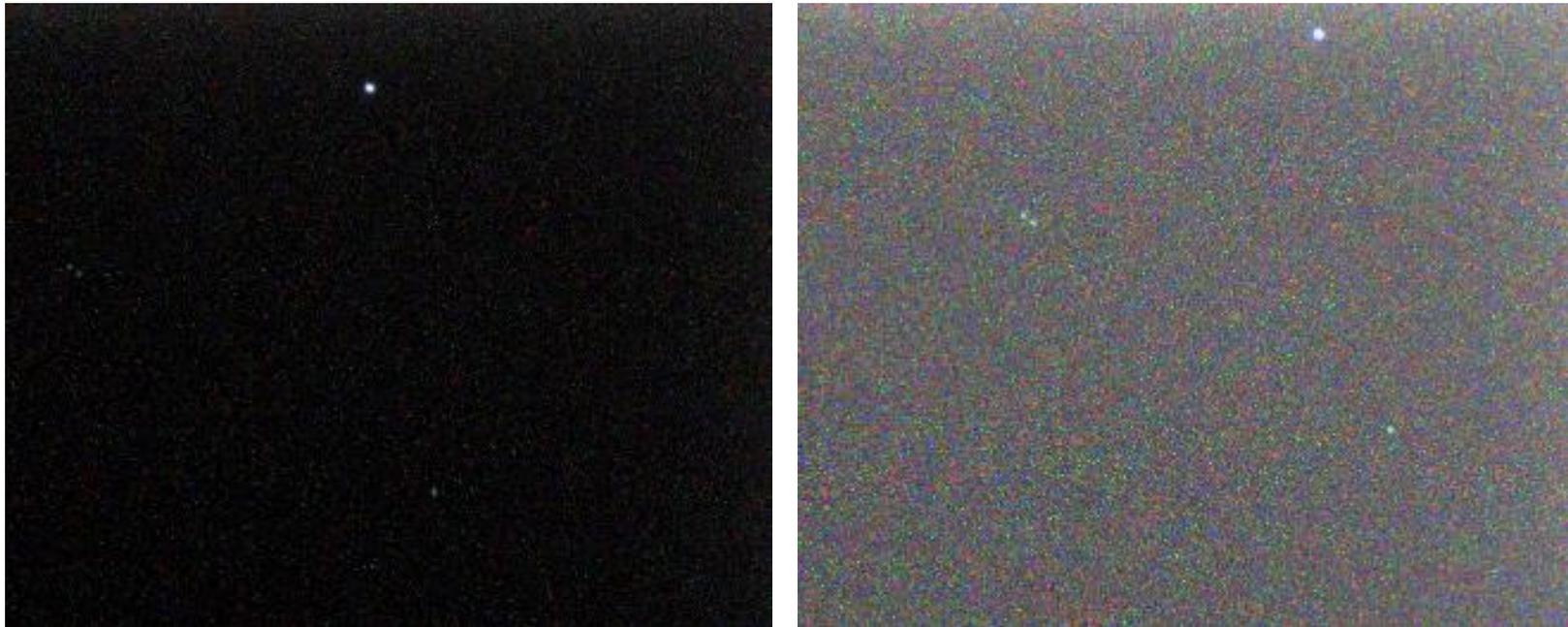
Captured unprocessed images during ground test of camera with exposure time 900 ms and sensor gain 5 dB (left image) and 18 dB (right image), sensor temperature was approx. 27°C. Unprocessed images are affected by thermal noise and by the dark current, allowing to recognize only bright stars (Vega, Double Double and Nasr Alwaki in figures).
