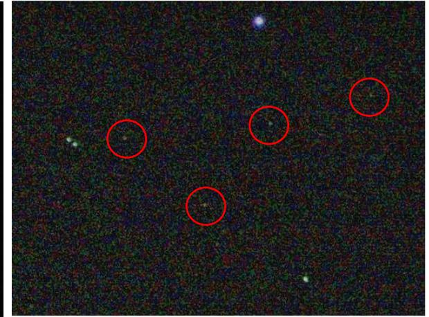
Gamma correction of previous image for better visualization of other recognized stars and residual thermal noise. Red circles show the newly recognized stars.
