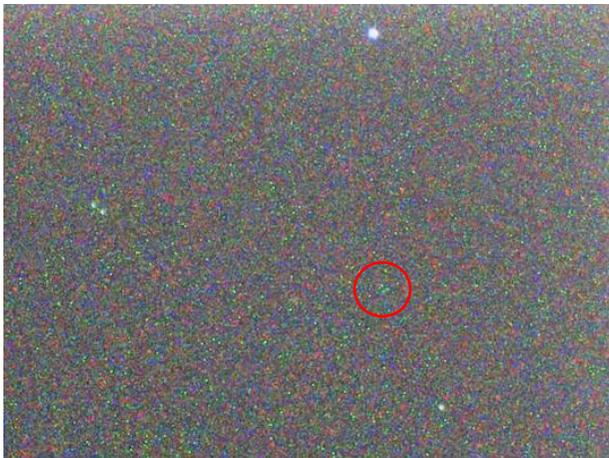
Cut-out of original captured image during ground test with exposure time 900 ms and gain 18 dB. Red circle shows hot pixels caused by the dark current, easily confusable with stars.
