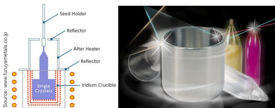
Only non-alloyed, very pure materials such as platinum, iridium and gold can be used for growing single crystals from oxide melts. The melting temperature, the atmosphere and the constituents of the melt determine the choice of material. Iridium crucibles are used at temperatures up to approximately 2300° C for growing crystals of high melting oxides for laser technology and the optical industry. [3]
