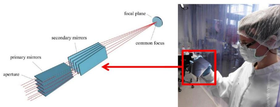
Iridium coatings promise excellent reflectivity properties in the X-ray range. Together with its international partners the coating laboratory at Aschaffenburg University is developing thin iridium reflection layers for space-based astronomical X-ray mirrors. [1] [2]
